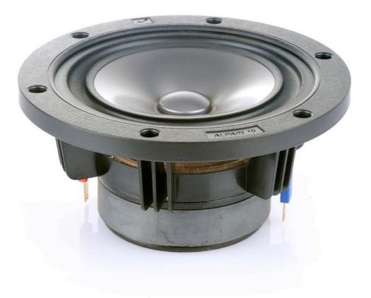
This Alpair 10 Gen.3 is the latest model in a development line designed to extend the performance of mid-sized Markaudio full-range emitters. This generation of Alpair 10 utilises a new ultra thin wall coil. Together with a further modifications to the cone, this latest model delivers usable frequency range up to 25-kHz while retaining its "purist" single cone design,
